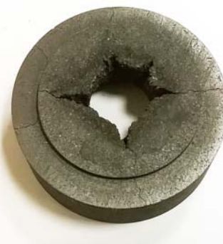
Fig. 3 – Eroding insert of nozzle critical section after fire test execution
