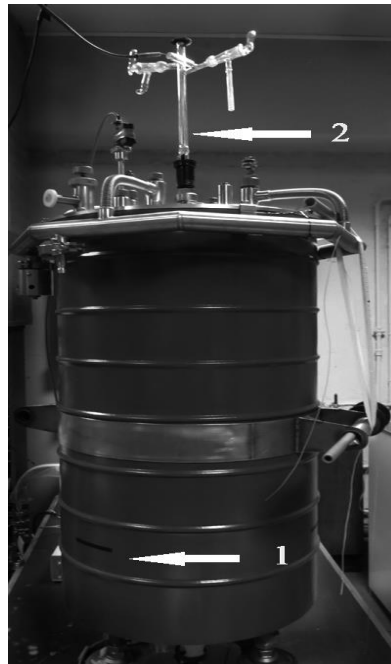
Fig. 1 – A general view of the cryostat with the cryomagnet; 1 – location of the centre of solenoid; 2 – glass discharge tube. The superconducting solenoid is in the bottom part of the cryostat, its length is 193 mm, the diameter is 146 mm, the diameter of the warm hole is 60 mm
