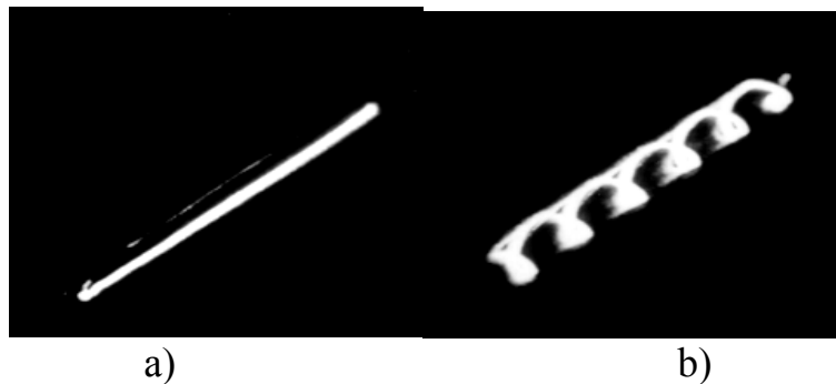
Fig.1 - Various trajectories of a cord discharge: a) discharge at a direct current; b) spiral structure in acoustoplasma
