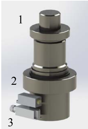
1 - LPRE; 2 - electrical field sensor; 3 - magnetic field sensor Fig. 4 – Deployment of alternating electrical and magnetic field sensors in proximity to LPRE
